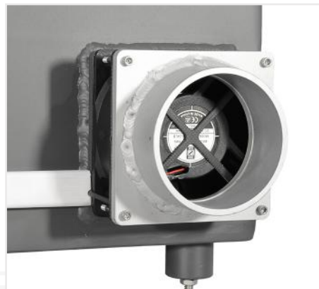
Outlet fan to evacuate gases after the test
