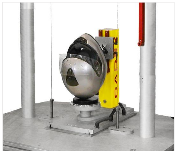
Shown installed on a Cadex twinwire impact machine
