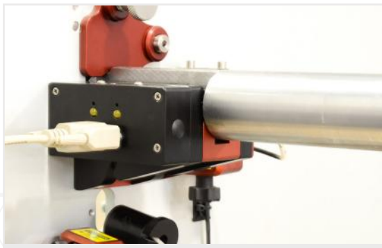
Easy removable timegate for periodical calibration
