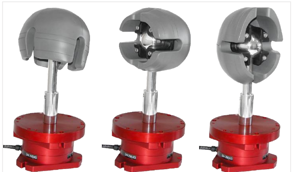
To be mounted on load cell with clamp - Available separately (P/N: 200_06_LCA3_22)
