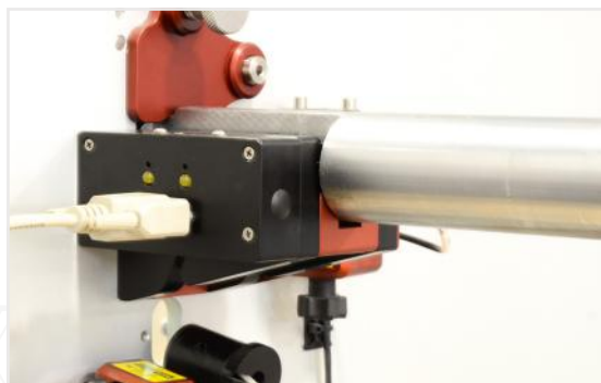
Easy removable timegate for periodical calibration
