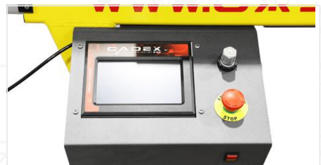
Touchscreen controller & pressure gauge
