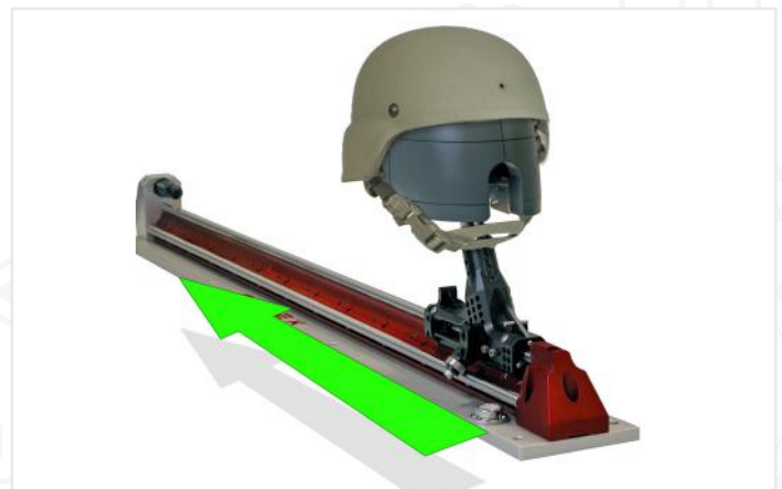
Shown during ballistic impact attenuation test
