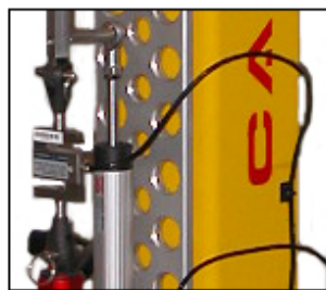
Double linear transducer and load cell incorporated.
