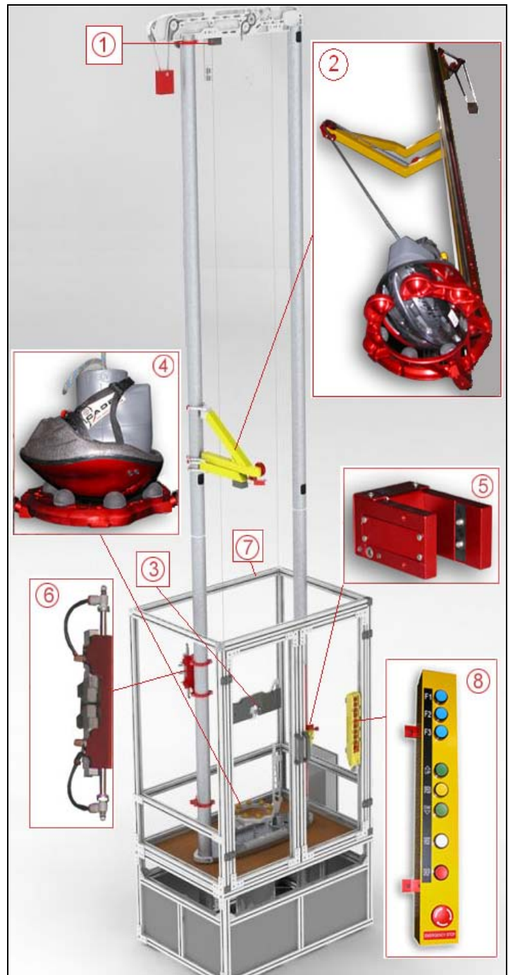
Twin wire system – Triaxial application
