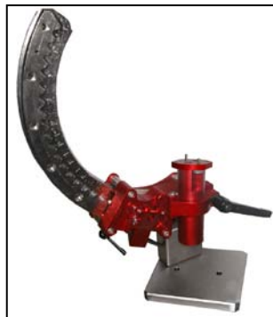
Rotates 90° vertically (every 5°) and 360° on its axis.
