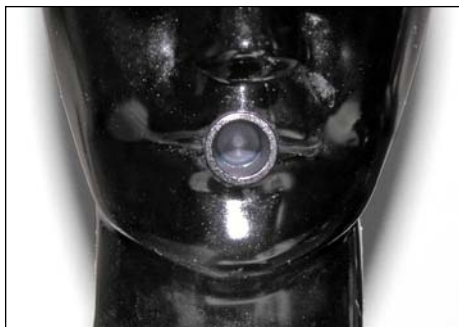
Breathing tube can be connected behind the headform or below the neck.
