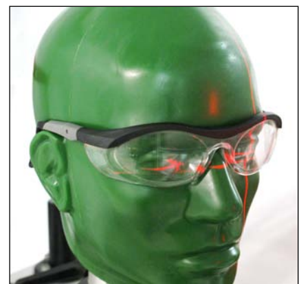
Alderson Headform during eyewear test. (Also available in green)
