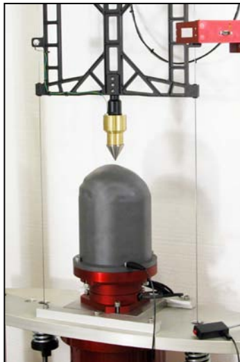
Shown performing resistance to penetration testing procedure.
