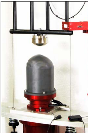
Shown performing shock absorption testing procedure.
