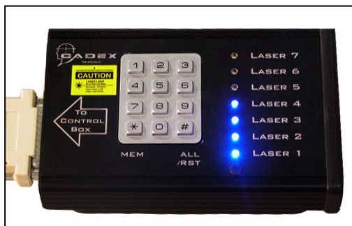
Led illuminated control box with numbered lasers.
