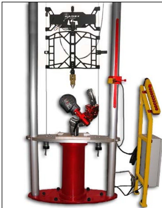
Penetrator installed on Twinwire.
