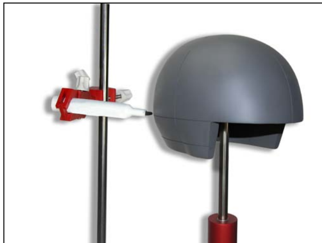
Traces precise markings on headform
